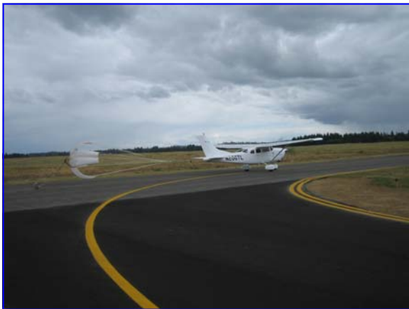
Soloy's engineering staff test the Cessna 206H Mark 2's recovery chute prior to exploring the spin characteristics of the new turboprop.
